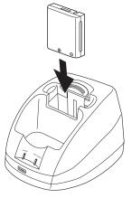
Note: Charge the Battery Pack without interruption for 12-15 hours.
